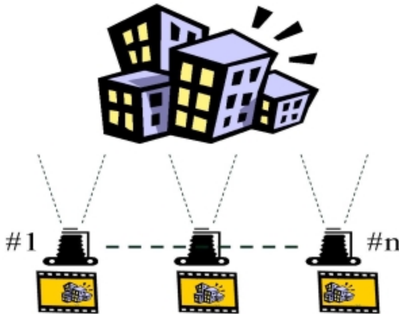
Figure 3. Image Creation. Multiple cameras, virtual cameras in computer space, or cameras in the visual world, are equally spaced along a straight-line, look at the scene or objects to be captured. These individual images, or tiles, are then Interziggled (see below) to produce the pixel map required by the SynthaGram lens sheet. The map contains the multiple perspective views.
